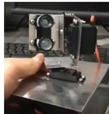
FIGURE 1. CONFIGURATION I ILLUSTRATING THE LIDAR-LITE V3 RANGEFINDER AND THE TOWERPRO SERVOS ON A BENT ALUMINUM BASE.
