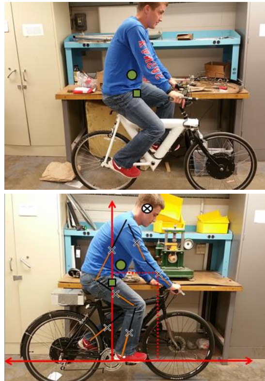
Figure 5. The method used to calculate the rider's COM for the first-year e-bike (top) and second year e-bike (bottom). The points marked by (x) are the COM locations of each body segment, the dashed lines were used to find their coordinates with respect the origin (placed at the bottom bracket), the solid circle is the COM of the rider and the solid square is the overall COM of the e-bike and rider.
