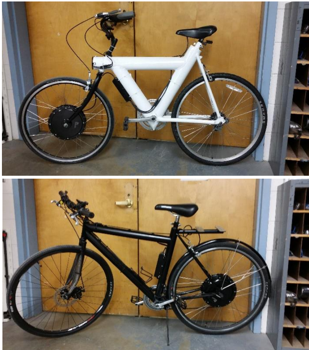
Figure 4. Both e-bikes were powder coated to improve their appearance with the first e-bike illustrated in the top image, and the second e-bike in the bottom image.
