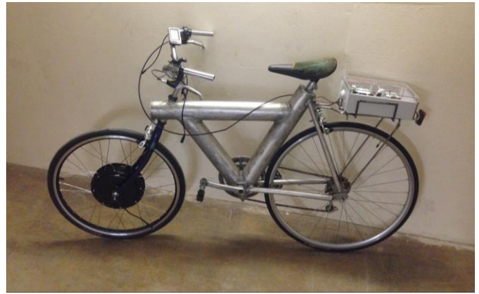
Figure 1. First year constructed e-bike including a rack to support the battery pack.
